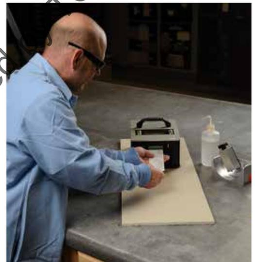
The new DCOF AcuTest (shown above) allows technicians to take accurate and repeatable measurements of DCOF thanks to an automated device, known as BOT-3000. This test replaces the manual ASTM C1028 method for calculating SCOF (shown below), which allowed too many variables into the process.
